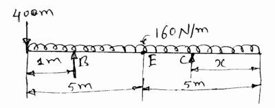
Determine the value if x, if the mid-point is a point of contraflexure and for this arrangement draw S.F. and B.M. diagrams.
